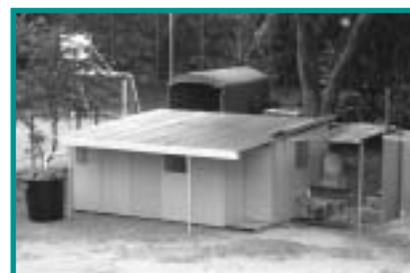
The temporary modular family unit is quick and easy to set up, can house a family of 5-6, and can be expanded by adding additional modules. The unit includes an ecologically safe latrine, shower and sink until a more permanent sewage system can be set up. Water tanks are included to capture rainwater.
